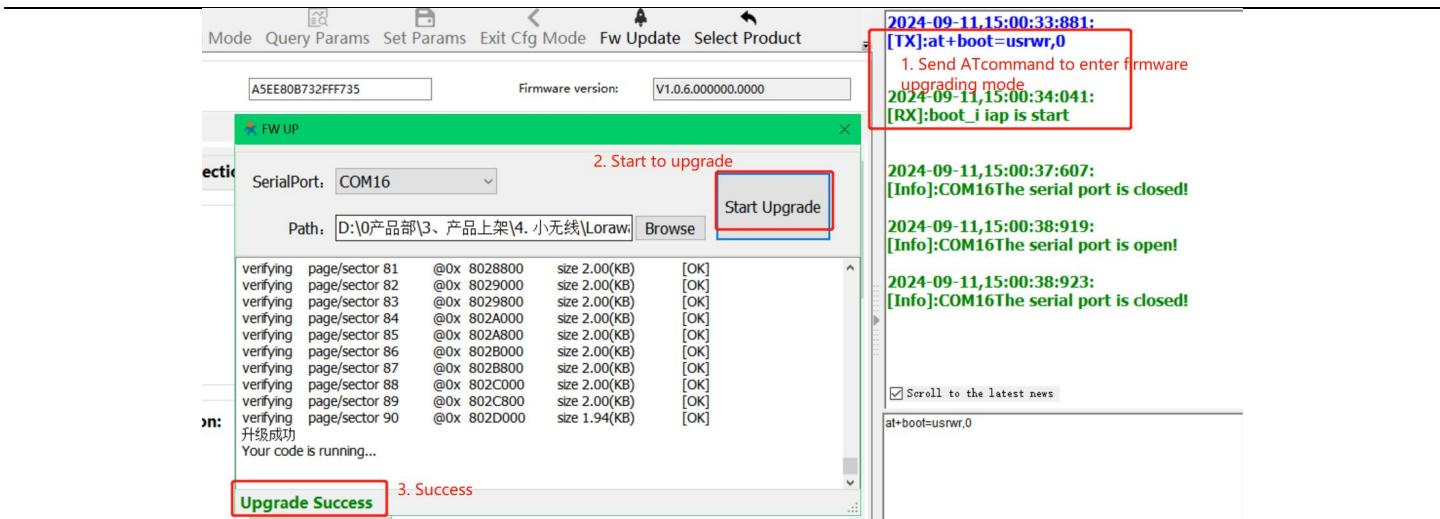
2. Press reload button, and then power on USR-DR206 device, then click the "Start Upgrade" button to upgrade.
