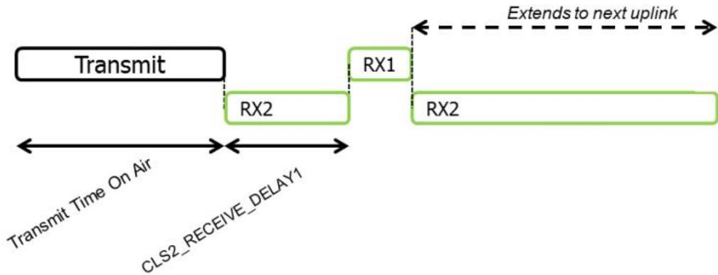
➤ Data Rate: The data rate of the RX1 window is typically one less than the uplink data rate. For instance, if the gateway's LoRa channel is set to DR5, then the data rate for our node's RX1 window can be set to 4. Refer to the data rate table for details.
