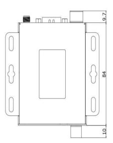
Sheet metal shell, fixing holes on both sides;
